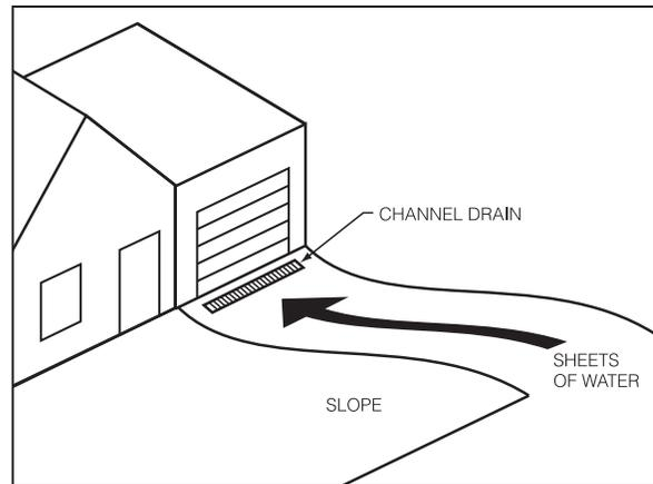
**Figure 4-3: Trench drainage**
